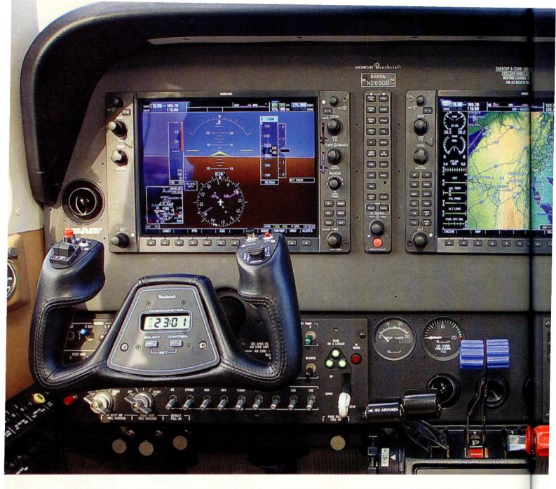
Much has changed with the Baron even if the name's been the same since 1961. The engines have swelled from Continental IO-470s rated at 260 horsepower to today's 300-hp Continental IO-550s. The maximum gross weight also has climbed 620 pounds to the current 5,500 pounds. The fuselage was stretched in 1970 from the original fourpassenger version to six total seats. The 1970 model was designated the B58 and is largely the same airframe that is produced today.
